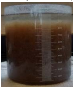
Figure 4: Sludge Volume Index Test Before BIO GENESIS® application SVI on 7/20/2015
