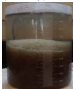
Figure 4: Sludge Volume Index Test Before BIO GENESIS® application SVI on 7/20/2015
